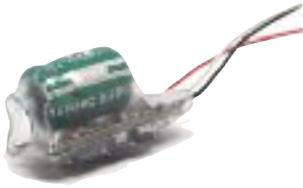
The Train-O-Matic Smart Powerpack (SPP) is compatible with all Train-O-Matic Lokommander II decoders, as well as with third party brands that have an energy buffer connection with three wires: U+, Masse/GND (Ground) and Charge. This includes ESU and Lenz. The manual that belongs to this Smart Power Pack will explain you how this Powerpack works in general and how to connect it to Train-O-Matic decoders. It can be downloaded here:
